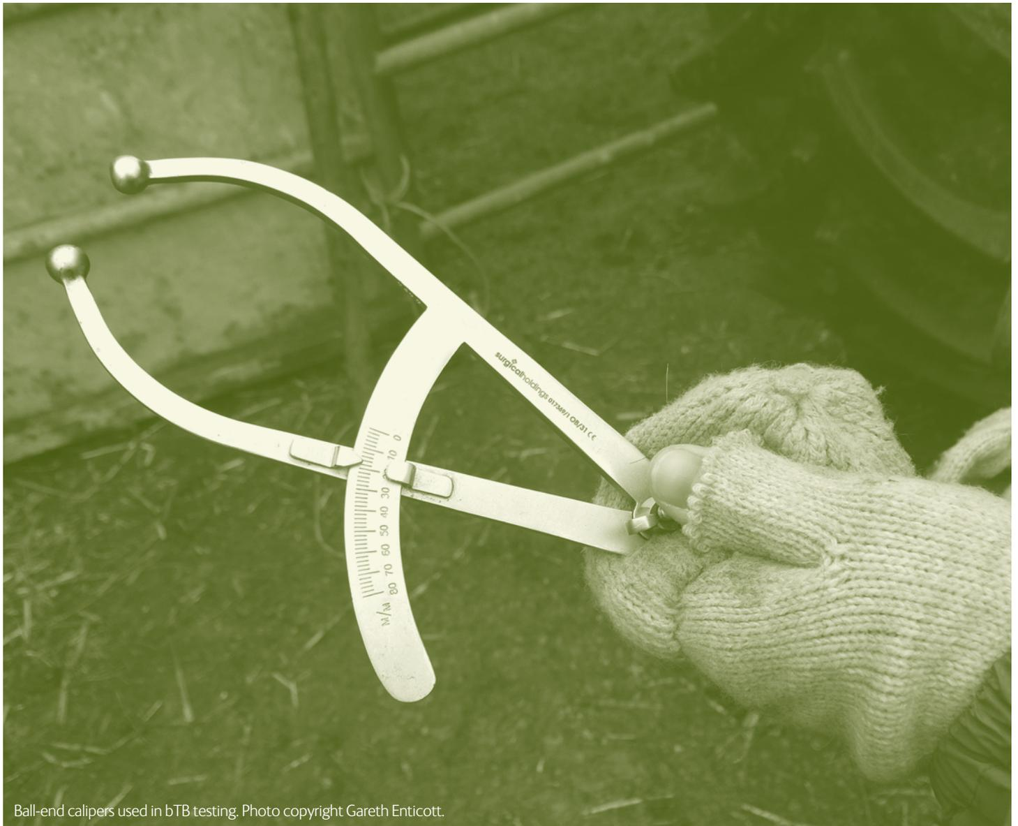
Ball-end calipers used in bTB testing. Photo copyright Gareth Enticott.
